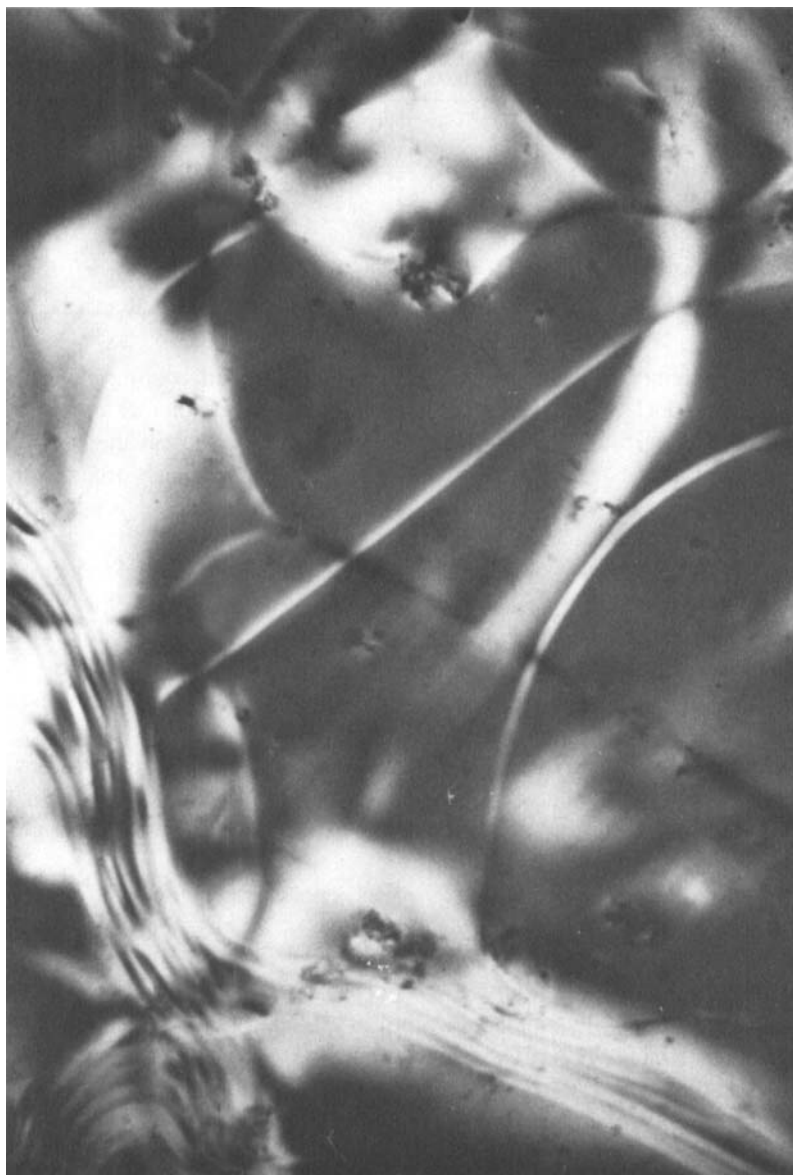
FIGURE 2 Photomicrograph of edge of broad planar region of a PBLG (MW = 130,000) liquid crystal 20.6% wt/vol in a 75:25wt% mixture of DCA and DCE.
